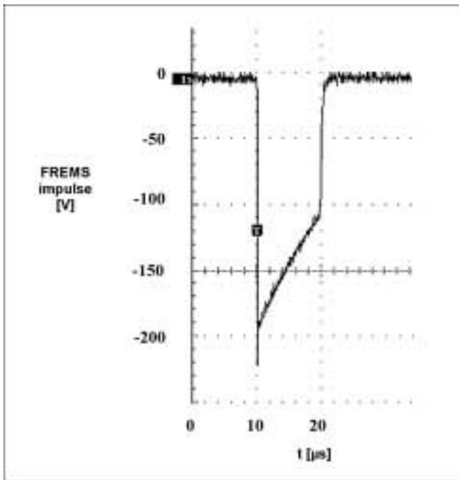
Figure 1.—Single pulse of the frequency rhythmic electrical modulation system (FREMS) sequence. This image was obtained from a high resolution oscilloscope connected with the output of the FREMS device (APTIVA., Lorenz Biotech S.p.A., Medolla, Modena, Italy). Voltage is expressed on the ordinate (50 V per division), time on the abscissa (10  $\mu$ s per division).
